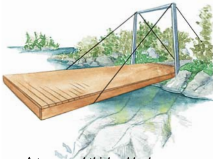
A tower and thick cables keep a suspension dock up in the air.
